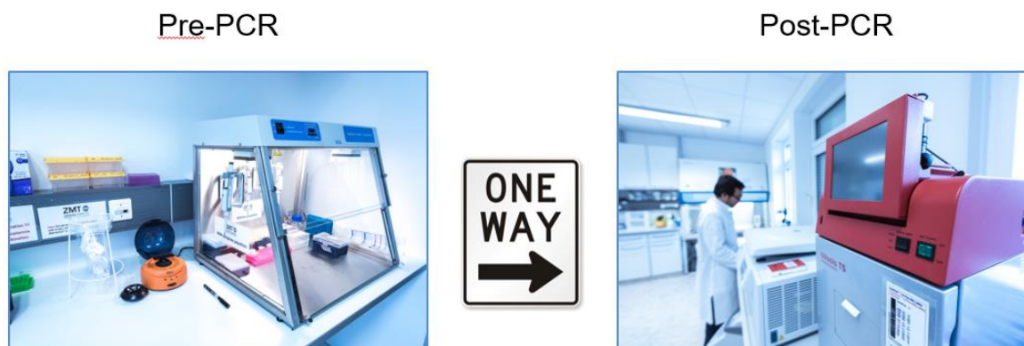
Figure 6: Spatial Separation of working areas in different rooms at ZMT (photos Tom Vierus). Left: Pre PCR lab with UV hood to set up PCR reactions. No genomic DNA is allowed within the hood, but the extraction area is in the same lab but on another bench. Right: Post PCR lab with gel documentation. No transfer of any equipment from Post-PCR to Pre-PCR. Be careful with your lab book and lab coat as well.
